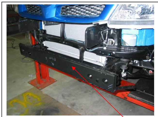
Figure 1 Remove original cross member
