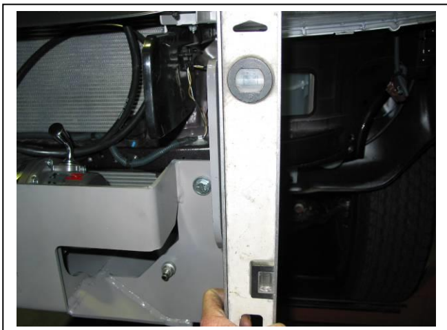
Figure 25 – Shown levelling passenger side steel mounting bracket off side
