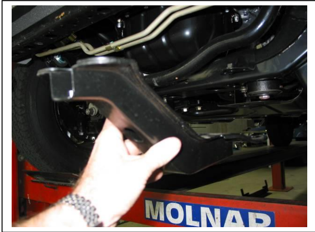
Figure 9 – Shown removing cross member supports
